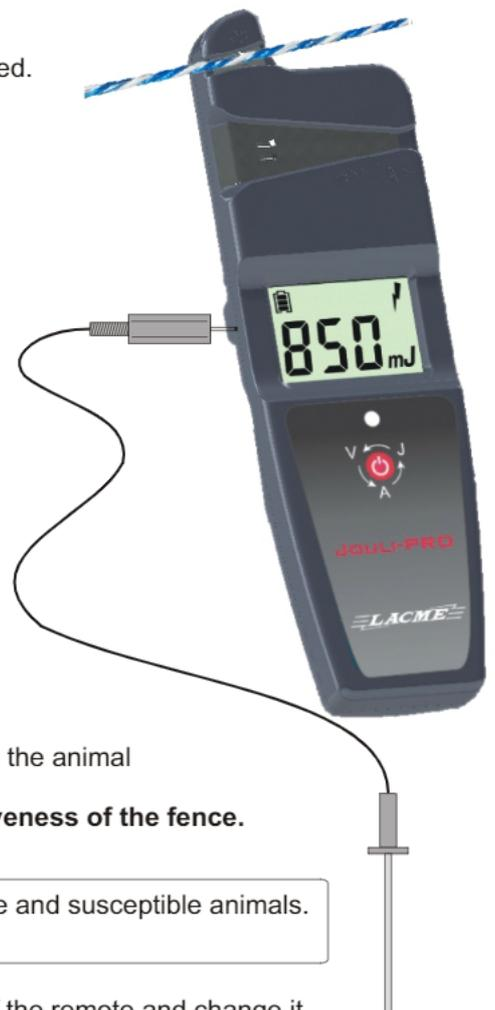
To change the battery (if indicator
