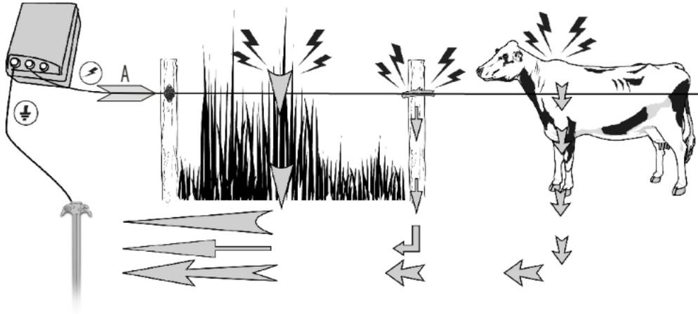
The current leaves the energizer, and circulates through the conductor looking for any way possible to return to earth. The return to the earth can be done via the grass, faulty insulator, animal touching the fence, etc ... The digivolt measures the importance of the current flowing through the conductor (A). And the arrow indicates the direction of current flow.
